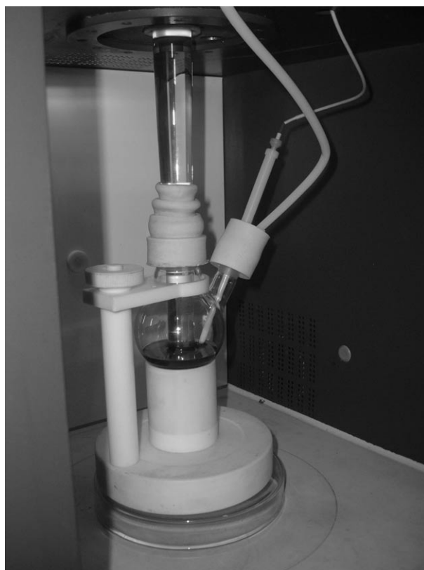
Figure 1. Standard set-up for simultaneous MW/US irradiation.
